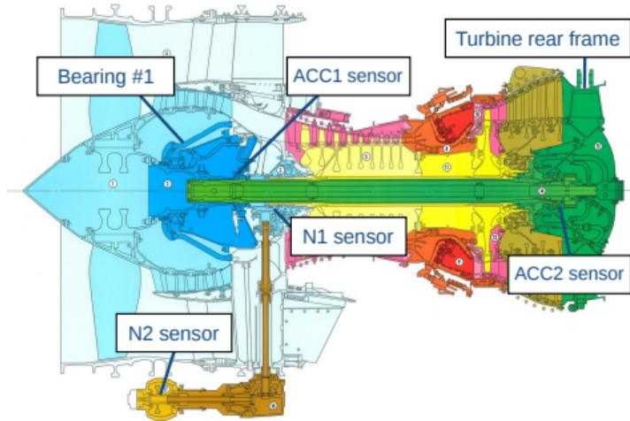
Sensors measure rotation speeds and vibration peak amplitude (displacement, speed or acceleration). Raw signals are processed and downsampled onboard.
